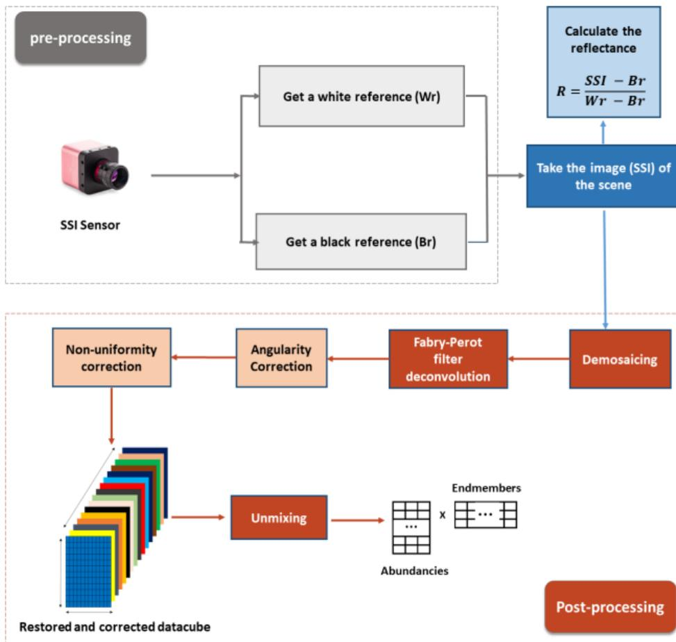
Assuming a Linear Mixture Model (LMM), deconvolution can be performed either before or after unmixing.
